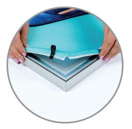
1) Start by folding one corner edge of the fabric so the silicone strip points down and the fabric wraps over it.
